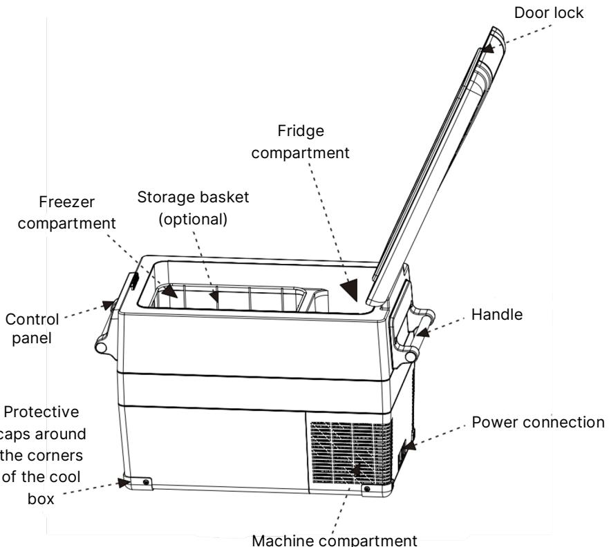
\* The temperature of the small compartment changes with the large compartment, only the large compartment can be adjusted, and the small compartment is usually used as a refrigerator that keeps food not to be frozen.
